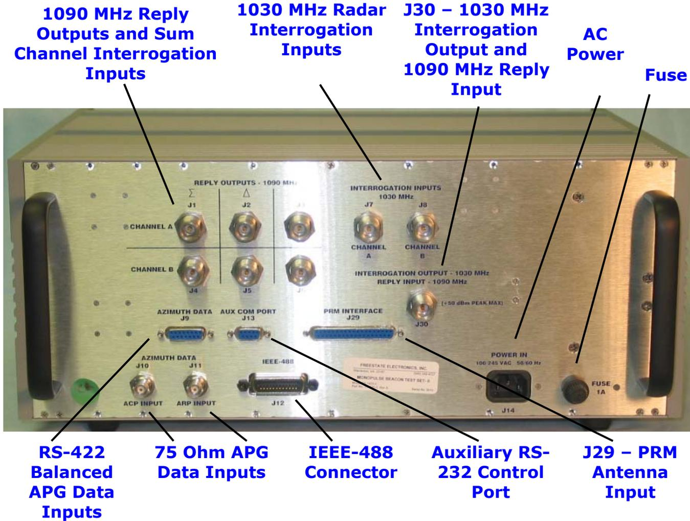
**Figure 41 PCC Module Front Panel Connectors**
