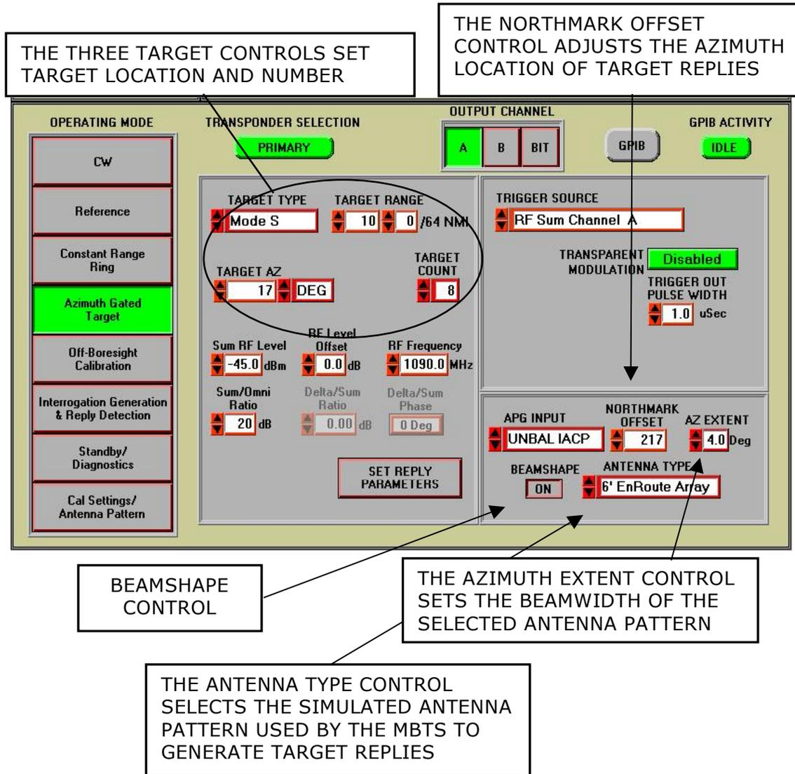
**Figure 33 Azimuth Gated Target Mode Function Block Diagram**
