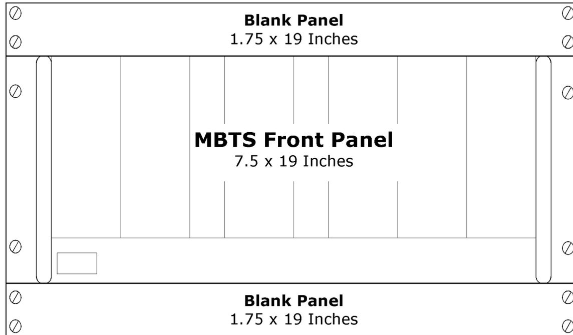
The MBTS front panel is 7.5 inches high, but a minimum opening of 10.5 inches is recommended for mounting it into an equipment rack. As shown above, 1.75 inch high blank panels should be mounted above and below the chassis to allow adequate air flow through the MBTS.
