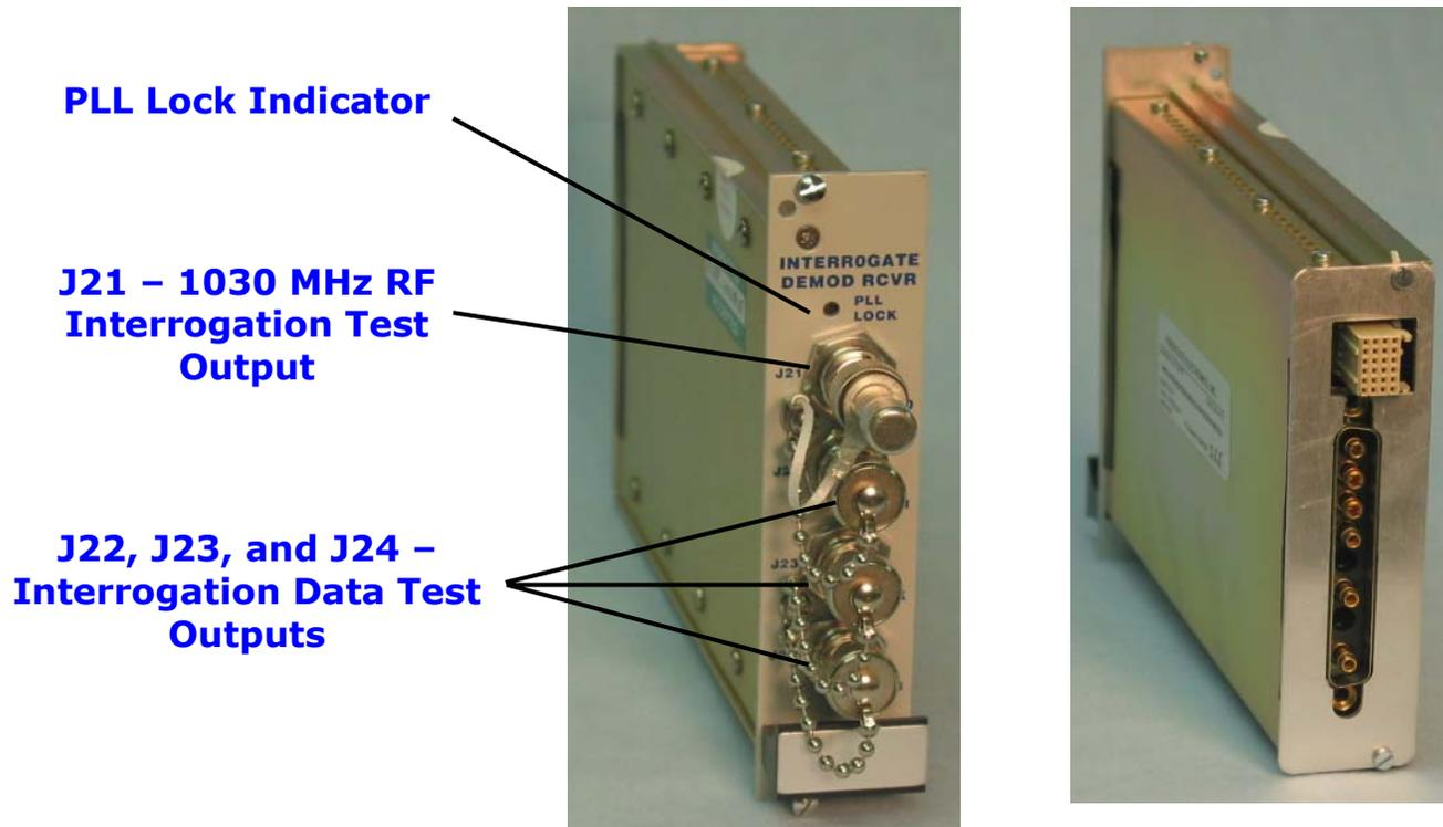
**3.4.1 J21 – 1030 MHz RF Interrogation Test Output**
