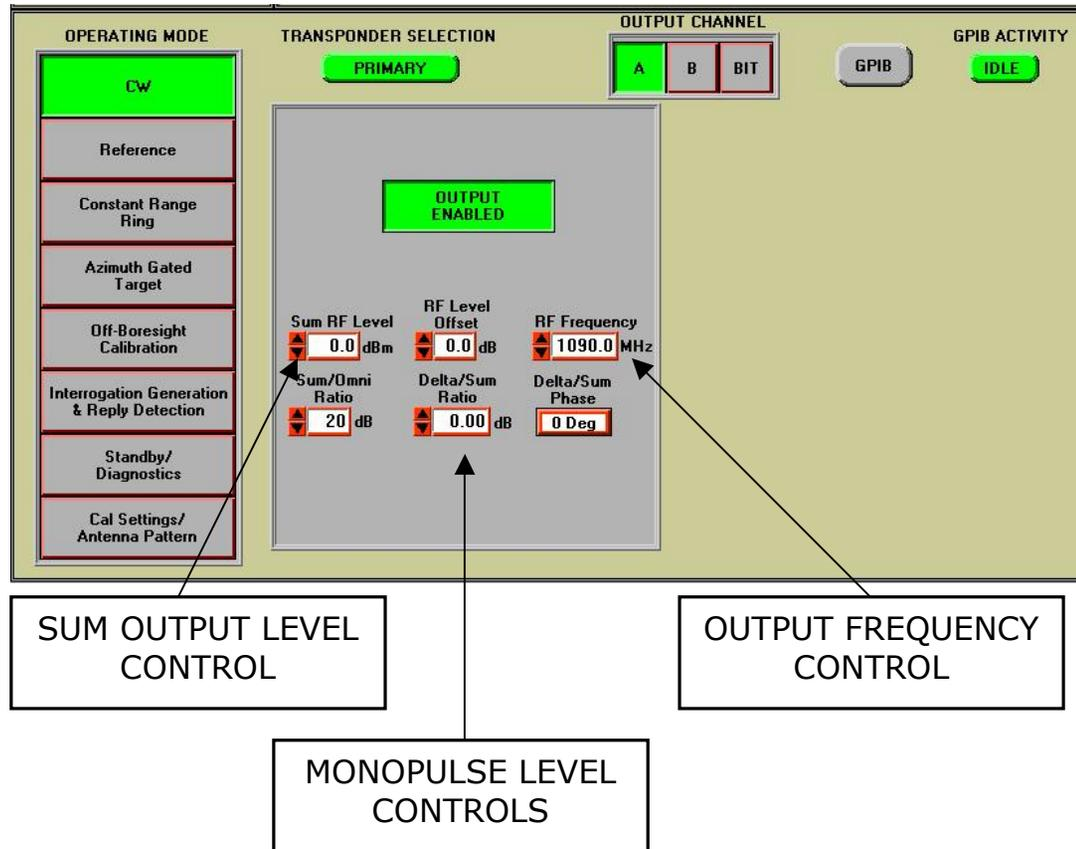
**Figure 27 1090 MHz CW Mode Control Functions**
