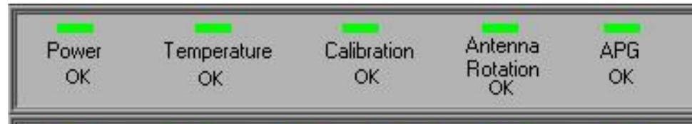
**Power Alarm:** Power Supply Status. ***Do not operate the MBTS if this alarm is red.*** See the [Power Supply and Chassis Temperature Panel](#).
