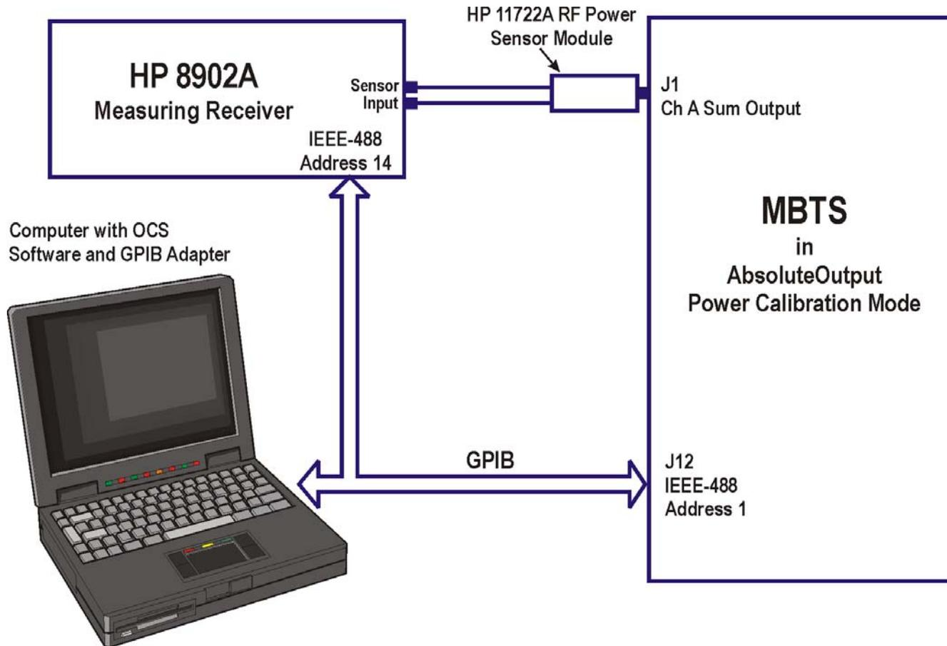
**Figure 1. Absolute Output Power Calibration Test Setup**
