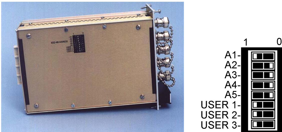
**Figure 2. PCC Module Side View Showing Setup Switches and Detail**
