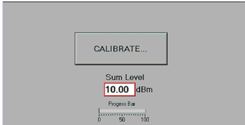
2. Click on the Calibrate control to start the measurement and calibration file generation process. If old calibration files exist, rename and save the old files in an appropriate folder or location on the OCS computer for archival purposes prior to starting the calibration process. Each old file should be renamed to include the serial number of the MBTS unit, as well as the date and time of the old file, within the new filename.
